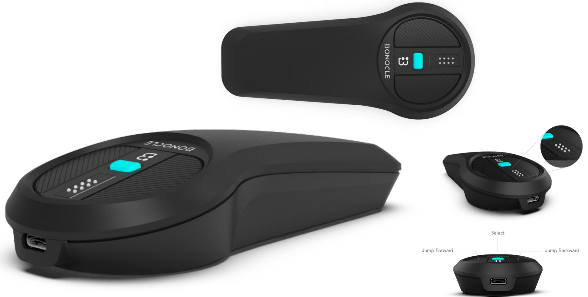
under the fingertip of the user when held or worn. The product is able to communicate with various electronic devices (e.g. smartphones, tablets, laptops or personal computers) and display the contents of the device in braille on the incorporated braille cell, providing the user with unprecedented access to the digital content available.
